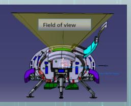
Late access doors located on vehicle either sides to allow loading of Payloads until 24 hours before launch
