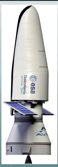
**Objective:** To provide a reusable orbital customizable/standardized system for multiple applications (microgravity, Earth observation, science, robotic exploration), integrated with Vega-C, able to perform inorbit payloads operations, de-orbit, re-enter, land on ground, be relaunched after limited refurbishment
